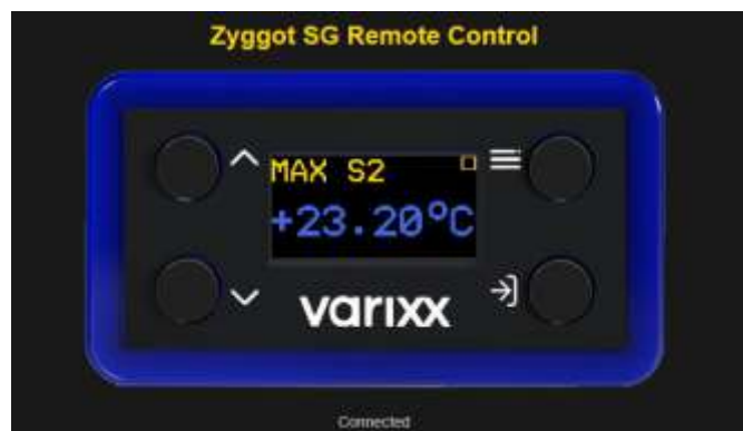
REMOTE CONTROL AND DATA READING BY ETHERNET
