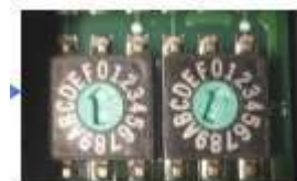
Address Rotary Switches for CAN at Eblock 88x from 1 to 253 (decimal) or 01 to FD (Hexadecimal)
