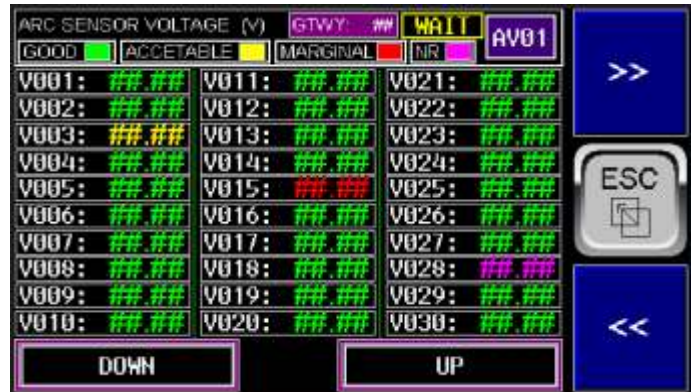
ARC SENSORS VOLTAGE LEVEL AV01 a AV04:
