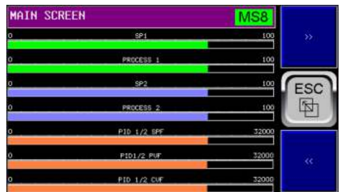
MAIN SCREEN MS8: Shows 7 bargraphs - bars of values from 0 to 100% or 0 to 32000
