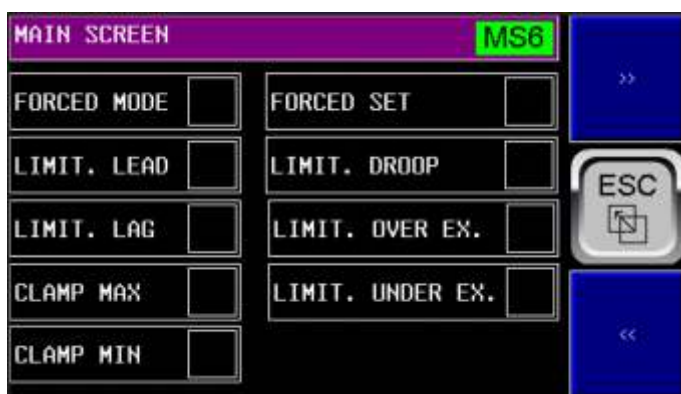
MAIN SCREEN MS6: Shows 9 fields of limiting, forcing and clamping conditions.
