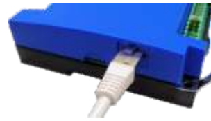
Detail of the RJ45 connector for communication with the relay (CAN)
