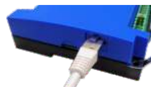
Detail of the RJ45 connector for communication with relay (CAN)
