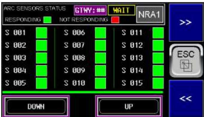
NOT RESPONDING NRA1 a NRA7: (Mono e Multi Gateway) Acessadas ao se pressionar <ARC SENSOR NOT RESPONDING>
