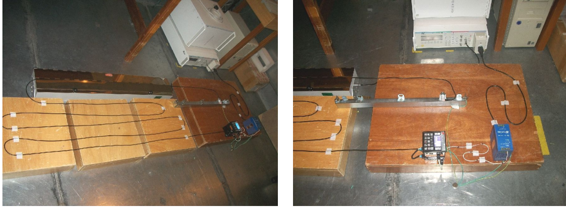
Photos 19 and 20 - Immunity to Electrical Fast Transient/Burst
